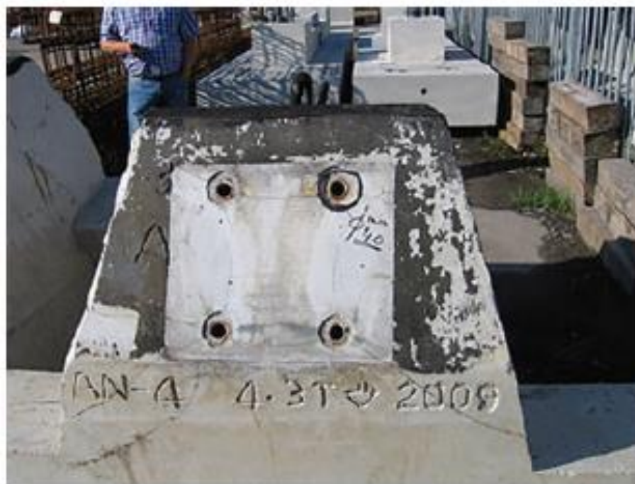
Figure 9: Damaged block due to the corrosion of anchor induced by stray current.
