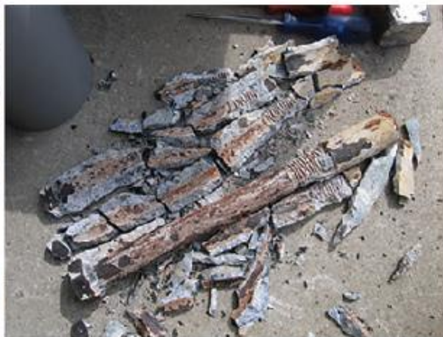
Figure 9: Damaged block due to the corrosion of anchor induced by stray current.
